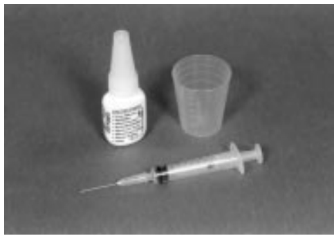
Figure 3 Medicine pot, needle and micropipette for dispensing the glue.
