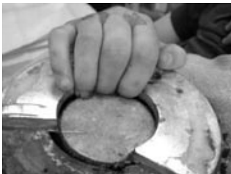
Figure 1 Fingers trapped in the magnetic gap (0.6 cm).
