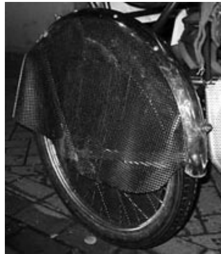
Figure 3 Protected spokes on the wheel of a modern recreational rickshaw.
