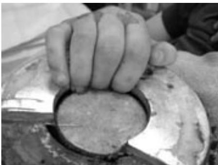
**Figure 1** Fingers trapped in the magnetic gap (0.6 cm).
