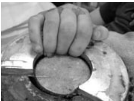
Figure 1 Fingers trapped in the magnetic gap (0.6 cm).
