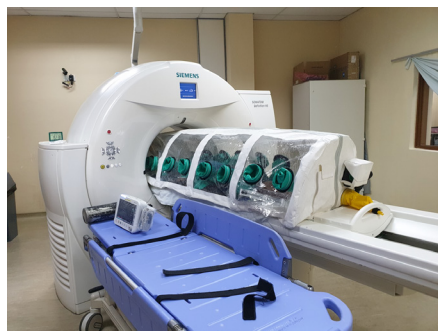
Figure 1 Negative pressure individual isolation system fitting comfortably into the CT scan gantry.
