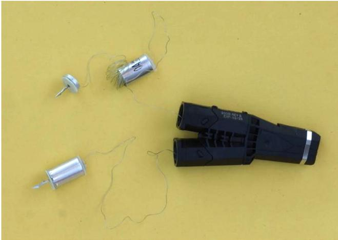
**Figure 3** TASER 7 probe separated (upper) and intact (lower).
